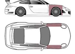
The mounting position of the transponder of a rechargeable or direct powered transponder is the same. The position must be identical on all cars competing in the championship. Fix the transponder vertically, at a maximum of 60cm (2ft) above the track. Make sure that the transponder has a clear view to the track with no metal or carbon fibre underneath. Maximum operating temperature should not exceed 122F/50°C.
