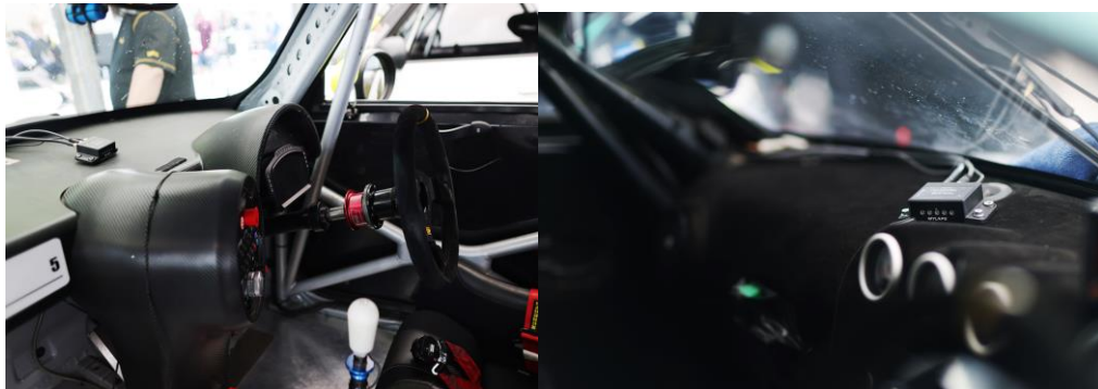
Installation examples (preferred position above the dashboard so that the driver can see the LEDs)
